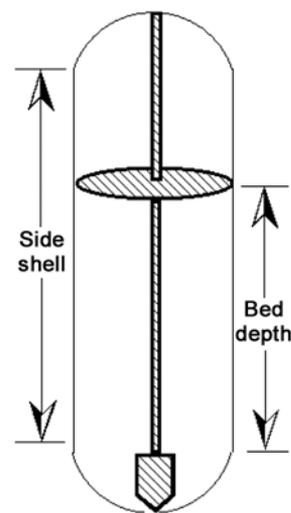
during backwash make sure that the freeboard (open space between the top of the media bed and the top of the tank) is greater than nine inches. It is common practice to leave 50-percent freeboard in media tanks. *Note:* Only use the side shell height (Figure 1) in calculating available freeboard and bed depth. If the media reaches the curvature of the tank during backwash, it is lost to the drain (see Figure 8).
